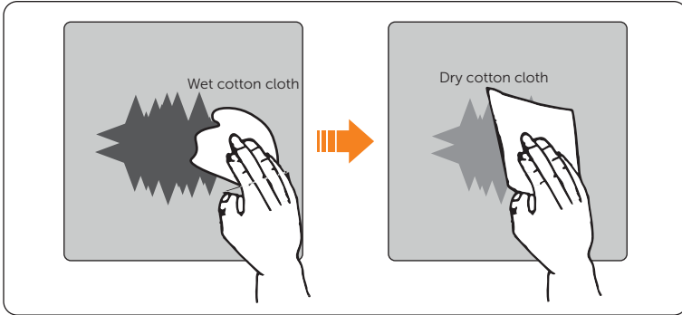
Figure 13-5 Cleaning the scratched area
